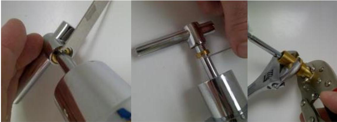
1. Disassemble your new Modern Lever taps with the anti-vandal spanner provided in the pack. It is **CRUCIAL** that you separate the Locking Nut from the Ceramic Cartridge as shown here.
